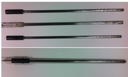
Fig. 7 The three pieces of the mandrel separated and combined
